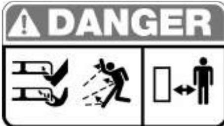
**WARNING!** SHARP PARTS. Keep hands and feet away. Do not operate the mower over gravel or foreign bodies which may be sucked up and ejected by the blades, generating a danger. Keep people away. Remove the key and read the instruction manual before attempting to carry out any maintenance or repairs to the machine.
