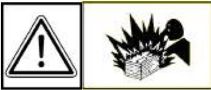
Prevent battery explosions: keep sparks, lighted matches and open flames away from the top of the battery. Battery gas can explode.
