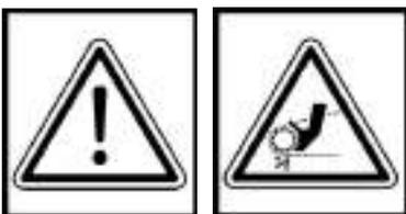
Caution! Never touch moving pulleys or belts. They can be very dangerous. Never do maintenance with engine running.
