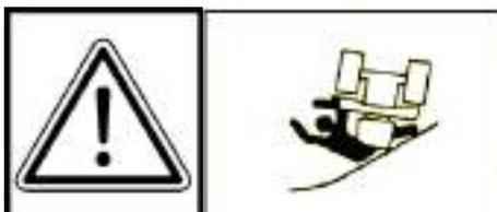
Avoid tipping. Do not drive where machine could slip or tip. Stay alert for holes and other hidden objects.
