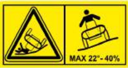
DANGER! Machine roll-over: Do not use this machine on slopes greater than 22° (40%).
